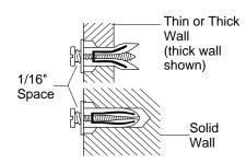
Figure 8 - Tightening Anchors
